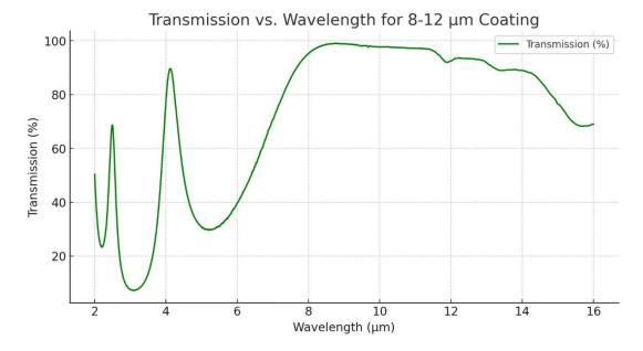
Typical transmission of a 3mm thick Ge window with BBAR (8000-12000nm) coating at 0° AOI. It indicates the coating design wavelength range, with the following specification:
