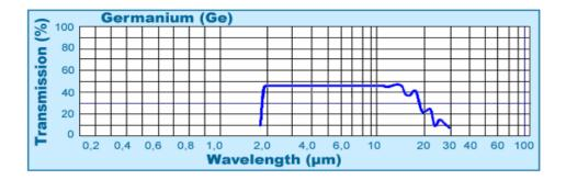
Here is the clearer plot of the typical transmission curve for a 1mm thick Germanium (monocrystalline) window. The graph shows a sharp increase to 50% transmission starting from 2  $\mu$ m and remains constant through 16  $\mu$ m. This graph provides a visual representation of how the transmission behaves across the specified wavelength range.
