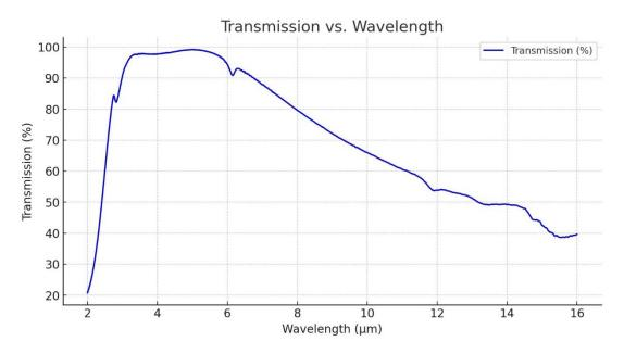
Typical transmission of a 3mm thick Ge window with BBAR (3000-5000nm) coating at 0° AOI. It indicates the coating design wavelength range, with the following specification:  $R_{avg} < 3\%$  @ 3000 - 5000nm
