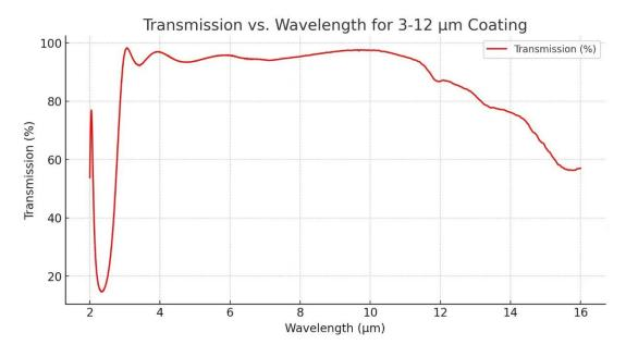
Typical transmission of a 3mm thick Ge window with BBAR (3000-12000nm) coating at 0° AOI. It indicates the coating design wavelength range, with the following specification:
